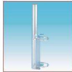
"FT-2" Fixing Bracket Top Size: \varnothing 38 mm for antenna fitting Bottom Size: \varnothing 45/50 mm for fitting on the mast Weight (approx.): 1100 gr Material: Galvanized Steel FT-2 Universal ..... 2510004.00
