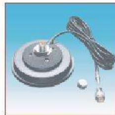
"HP MAG 125 PL" Magnet Mount Frequency Range: from DC to 500 MHz Materials: Nylon, Chromed brass, Teflon insulator, Gold plated pin, 3.6m RG58 C/U MILC17 HP MAG 125 PL ..... 2511202.05
