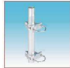
"FT-3" Fixing Bracket Top Size: \varnothing 30 mm for antenna fitting Bottom Size: \varnothing 35/54mm for fitting on the mast Weight (approx.): 350 gr Material: Anodized aluminium, Stainless steel FT-3 ..... 2511301.00
