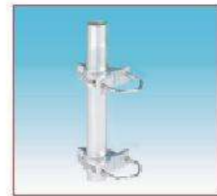
"FT-3" Fixing Bracket Top Size: \varnothing 30 mm for antenna fitting Bottom Size: \varnothing 35/54mm for fitting on the mast Weight (approx.): 350 gr Material: Anodized aluminium, Stainless steel FT-3 ..... 2511301.00
