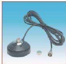
"HP MAG H 12 PL" Magnet Mount Frequency Range: from DC to 500 MHz Materials: Nylon, Chromed brass, Teflon insulator, Gold plated pin, 3.6m RGS8C/U MILC17 HP MAG H 12 PL ..... 2511802.05
