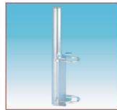
"FT-2" Fixing Bracket Top Size: \varnothing 38 mm for antenna fitting Bottom Size: \varnothing 45/50 mm for fitting on the mast Weight (approx.): 1100 gr Material: Galvanized Steel FT-2 Universal ..... 2510004.00
